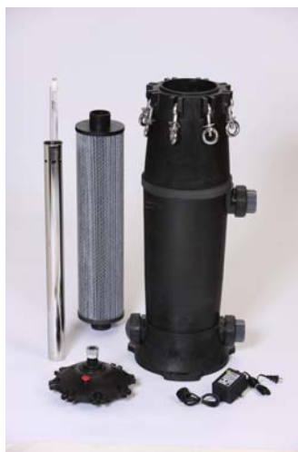
Components include filter housing, proprietary cartridge, stainless steel chamber, UV light, ballast, lid with swing bolt closure.
