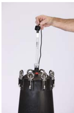
Lamps are easily replaced by disconnecting electrical power.
